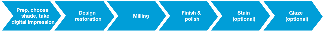
Figure 1: Overall workflow/procedure for preparing a restoration using a CAMouflage NOW Milling Block.
